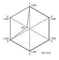
Test conditions: Shock is applied in  $\pm X$ ,  $\pm Y$ , and  $\pm Z$  directions three times each with without energizing the Relays to check the number of malfunctions.
