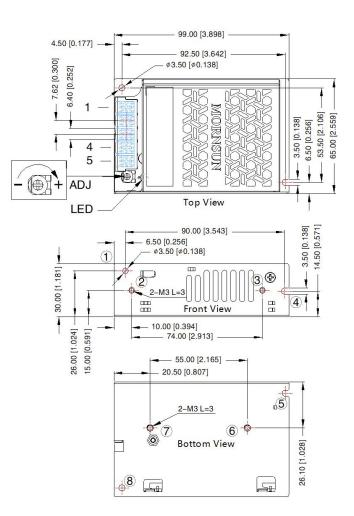
Pin-Out Pin Function 1 AC(L) AC(N) 2 3 4 -Vo 5 +Vo
